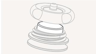
5 Connect the electrode cable connection to the fastener.
