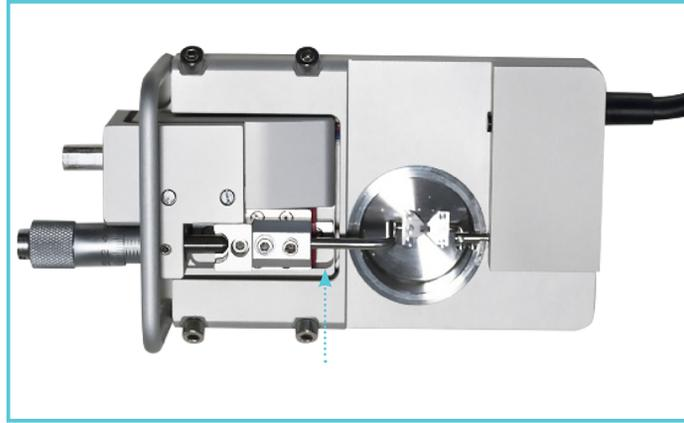
*Figure 4.5 Myograph unit - screws for changing supports and coarse adjustment of the jaws*
