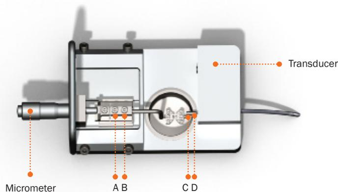
Figure 2.1 Illustration of the screws for changing supports and coarse adjustment of the jaws
