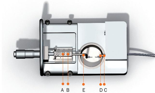
Figure 2.4 - Fine adjustments of the pins in the Myograph chamber
