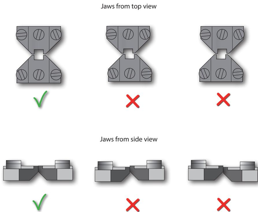
Figure 2.3 - Illustrations of properly aligned jaws (depicted on the far left) and incorrectly aligned jaws (depicted in the middle and far right).
