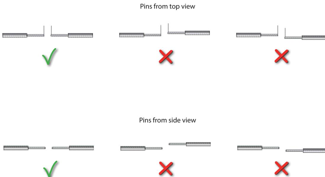
Figure 2.5 - Illustrations of properly aligned pins (depicted on the far left) and incorrectly aligned pins (depicted in the middle and far right).
