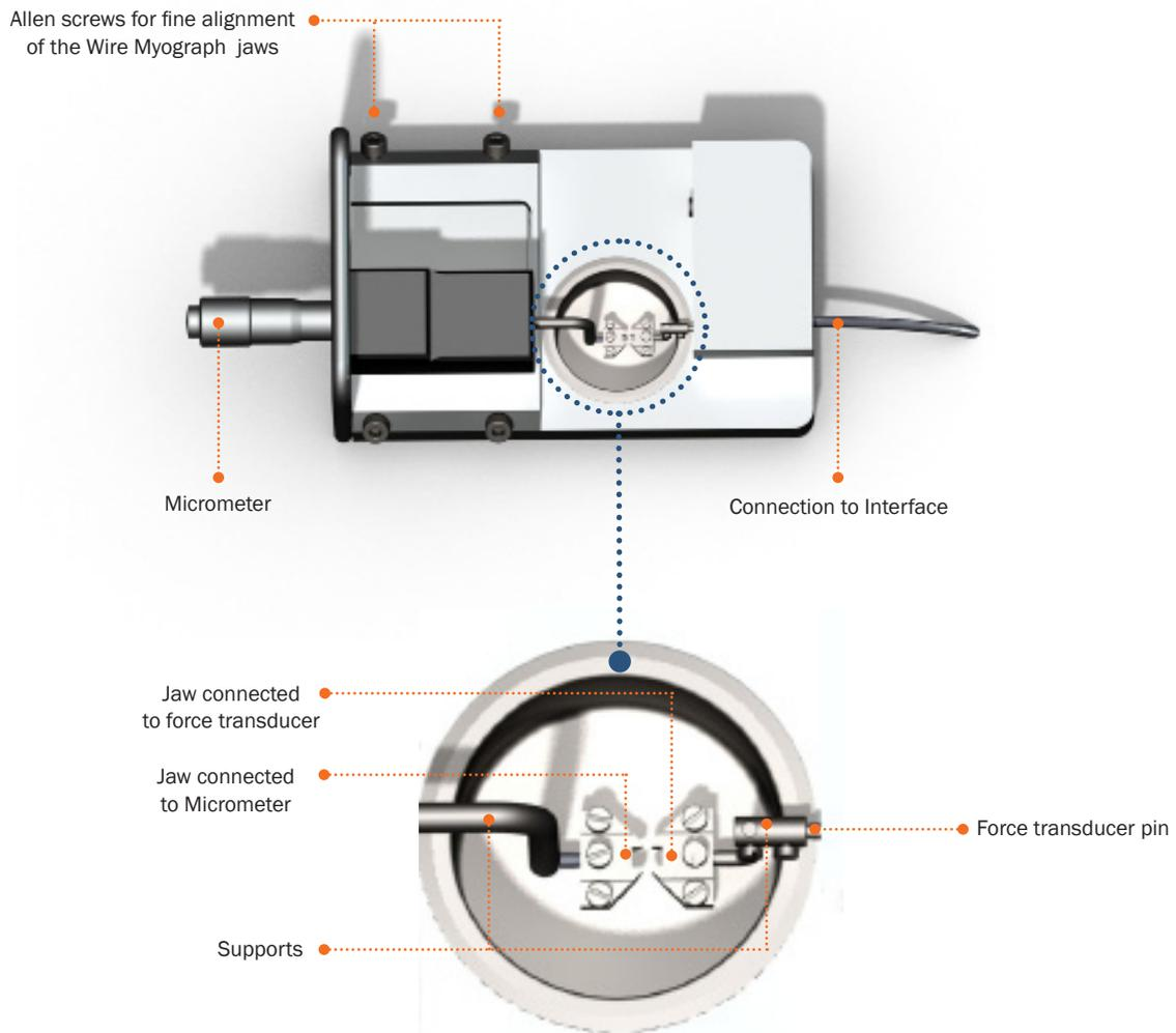
Figure 1.1 Wire Myograph with close-up of chamber
