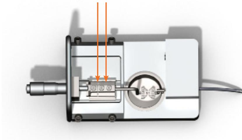
Figure 4.5 The areas where linear slide grease may be applied for smooth micropositioner movement
