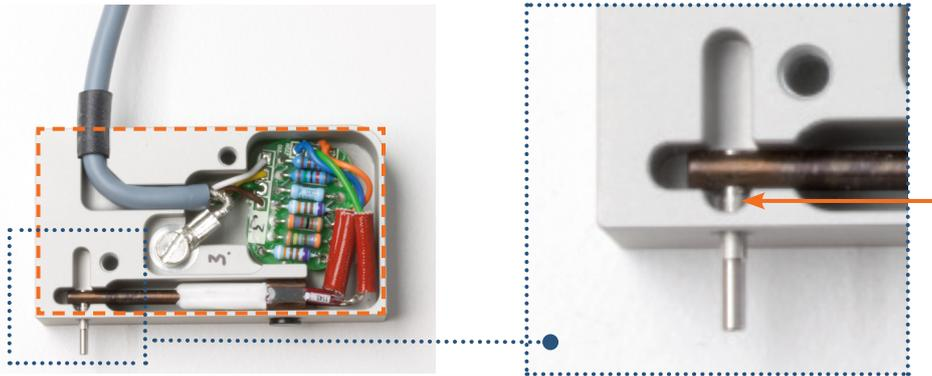
Figure 4.4 Inside the transducer housing and close-up of transducer pin.
